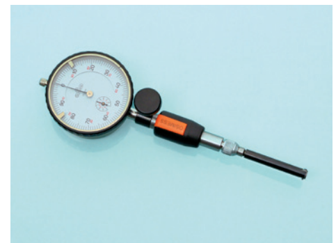
OSG measuring gauge for internal threads
